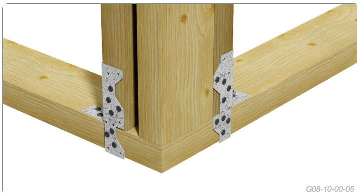
Studs to bottom plates
