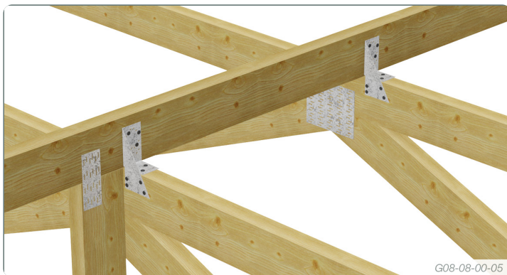
Jack flyovers to truncated truss
