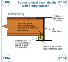
FLOOR: SJ Packer/Filler Block, SmartJOIST to SmartJOIST Fixing Details
