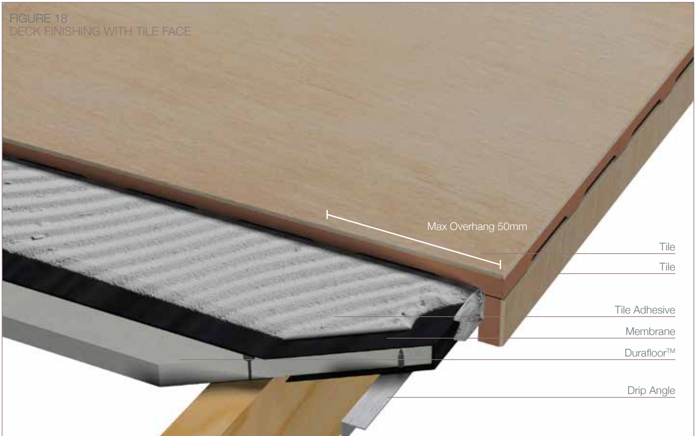
FIGURE 19 DECK FINISHING
